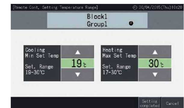
[Temperature Limitation for Each Remote Controller]
